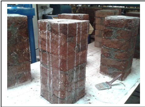
Figure 2 : Marking for FRP strips on Primer applied specimen
