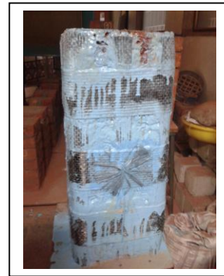
Figure 3 : CFRP with Anchors
