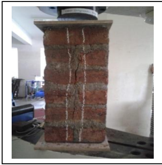
Figure 1 : Vertical Splitting Cracks
